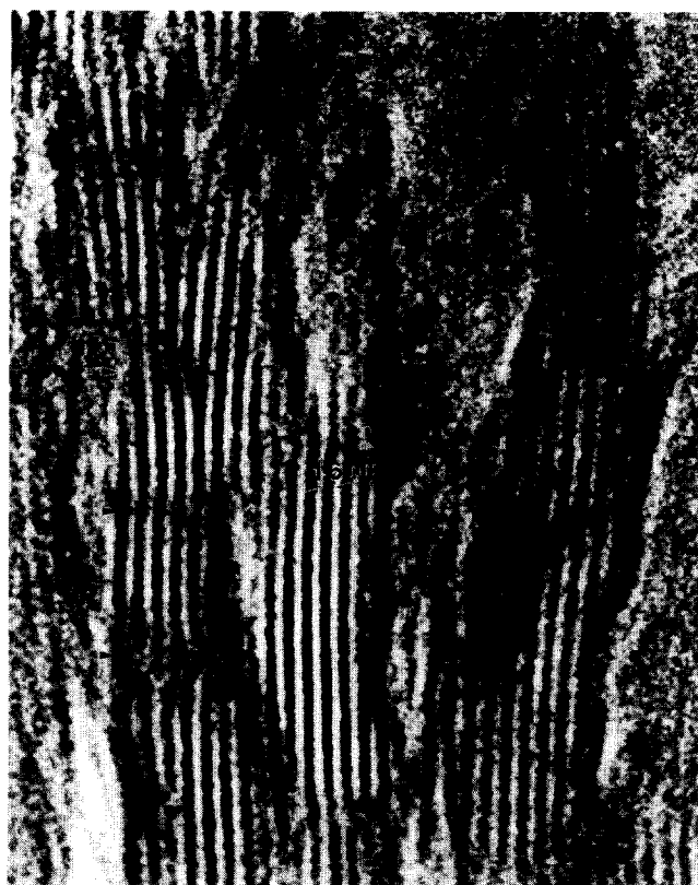
Figure 6 HREM image of PMDA-ODA lamellar crystals ([100] zone). The strong 1.6 nm (002) fringes correspond to the repeat distance from segment to segment along the chain backbone. The local orientation and perfection of the lamellae can be determined directly, and evidence for screw-dislocation-mediated branching is observed (arrows). Reproduced by permission from ref. 67
